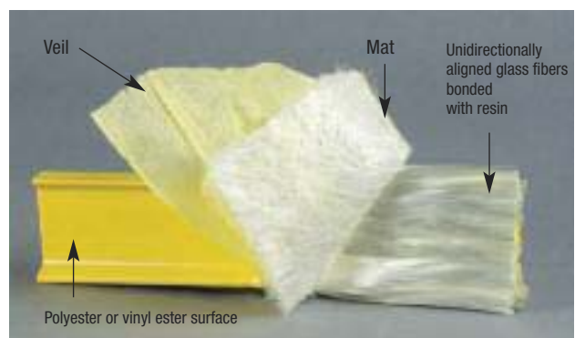
A surface veil is applied during the pultrusion process to ensure a resin-rich surface for superior corrosion resistance as well as an ultraviolet exposure barrier.
